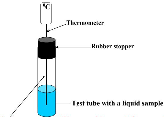
The thermometer should have a straight central alignment, with the central position of the thermometer's tip inside the liquid sample.
